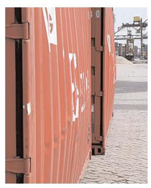
The International Standard Organisation (ISO) / Institute of International Container Lessors (IICL) deformation limit for sidewall panels is a maximum of 10mm beyond the plane of the side surfaces of the corner casting fittings.
