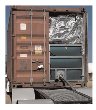
To ensure that a flexitank does not bulge through the gaps in a steel framework bulkhead a sufficiently rigid sheet should be placed on the inside of the bulkhead. This prevents the flexitank chafing against the steelwork. The photograph below shows horizontal steel bars used with cardboard sheeting placed between the flexitank and the steel bars
